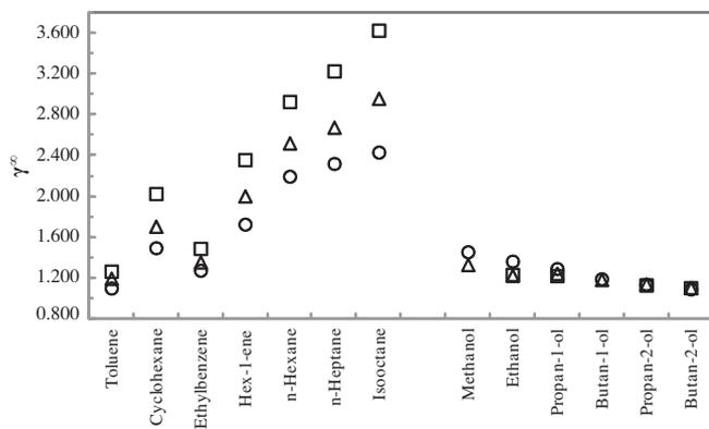
FIGURE 4. Plot of  $\gamma_{13}^{\infty}$  in linoleic (*cis,cis*-9,12-octadecadienoic) acid versus  $T$  for hydrocarbons and alcohols,  $\circ$  at  $T = 338.3$  K;  $\Delta$  at  $T = 348.3$  K; and  $\square$  at  $T = 358.3$  K.
