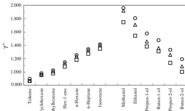
**FIGURE 2.** Plot of  $\gamma_{13}^{\infty}$  in stearic (octadecanoic) acid versus  $T$  for hydrocarbons and alcohols,  $\circ$  at  $T = 349.5$  K;  $\Delta$  at  $T = 358.4$  K; and  $\square$  at  $T = 368.1$  K.
