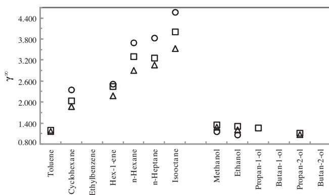
FIGURE 5. Plot of  $\gamma_{13}^{\infty}$  in linolenic (*cis,cis,cis*-9,12,15-octadecatrienoic) acid versus  $T$  for hydrocarbons and alcohols,  $\circ$  at  $T = 303.1$  K;  $\Delta$  at  $T = 313.3$  K; and  $\square$  at  $T = 323.3$  K.
